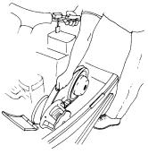
8. Firmly grasp the belt midway between the clutches and pull upward and rearward to remove. See illustration.
